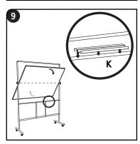
After the revolver is correctly assembled according to the supplied instructions, and after the revolver board is secured in it's place by the use of back knobs, the revolving functions of the revolver may only be used by loosenning both knobs, revolving the board to the desired face and tightning both knobs again. Failure to do so, may result in premature tear to the fixing mechanism.
